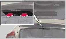
Pull release handles separately to fold left and/or right backrest.
